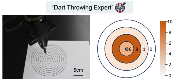
Fig. 5: Repeatability accuracy experience for AVR. We design a "dart throwing" test. After 50 demonstrations and 15 times deployment, results (right) show that 40% of the attempts had an error below 1 cm.
